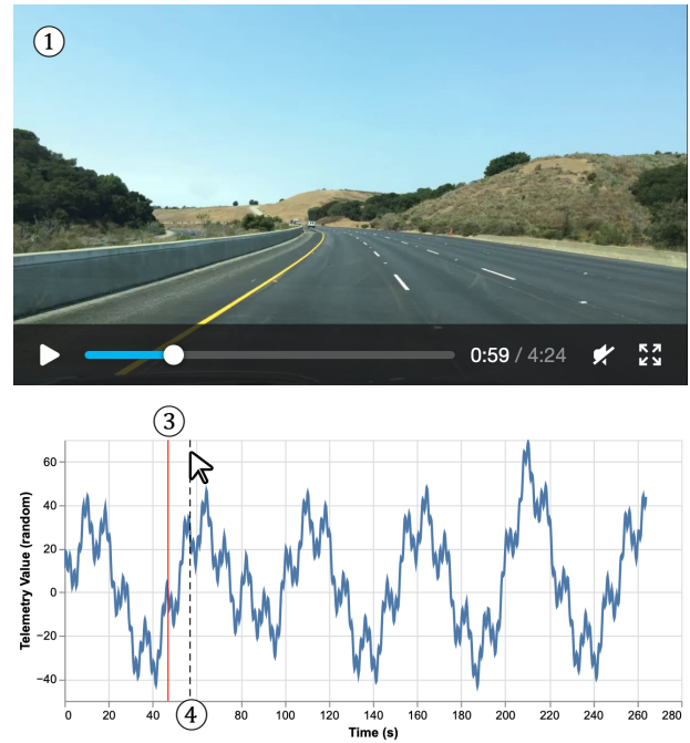
Figure 1: A partial Vega visualization syncing time series data with a video (①). Clicking or dragging on the plot updates the video's time (②). A red playback cursor, at 47s, displays the time of the currently presented frame (③). A dashed playback cursor, at 59s, displays the frame a user is targeting (④). Video frames in this and all subsequent figures from the BDD100K dataset [17] © 2018 The Regents of the University of California.
